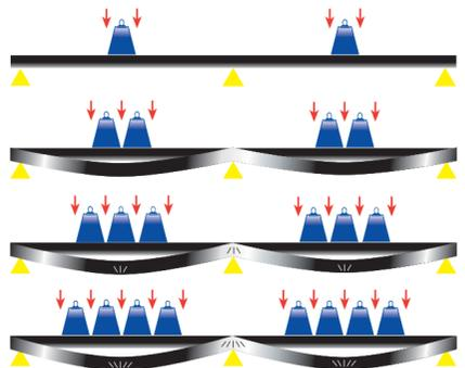
**"In general, the higher the steel ductility, the greater the ductility of the beam".**
