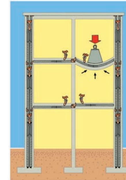
If we were in a building in an overload situation, for safety's sake, we would definitely prefer the structure to deform allowing us to evacuate, rather than to undergo a sudden collapse leaving us with no chance to escape in time.
